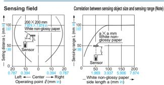
Note: As the sensing object size becomes smaller than the standard size (white non-glossy paper 200 × 200 mm 7.874 × 7.874 in), the sensing range shortens, as shown in the above graph. (For plotting the above graph, the sensitivity has been set such that a 200 × 200 mm) (7.874 × 7.874 in white non-glossy paper is just detectable at a distance of 100 mm 3.937 in.)
